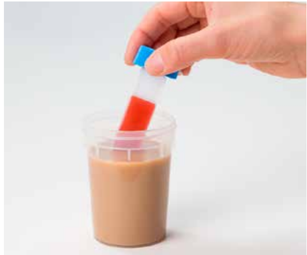
Use Easicult Combi to optimize the biocide concentration in cutting fluids.
