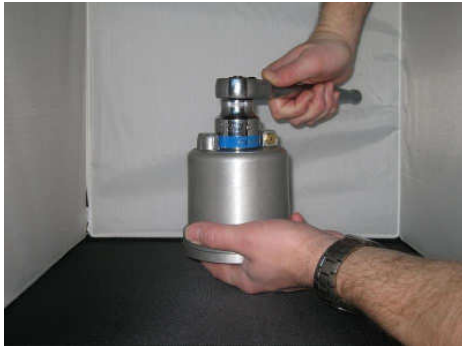
Hold Rotor in Hand and tighten Rotor Nut with Spanner
