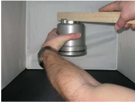
Tap Rotor Nut with Wooden Baton to separate Rotor parts
