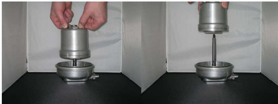
Block Jets with Fingers and lift from Rotor Shaft
