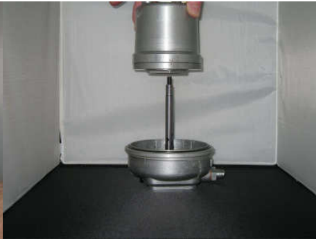
Slide Rotor onto Rotor Shaft
