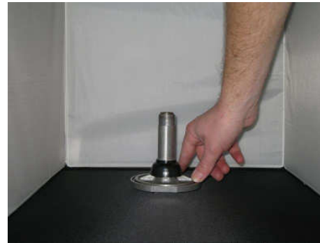
Reassembly Fit Rotor O'Ring
