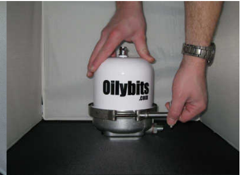
Fit Rotor Cover, Tighten Top Nut *Re Fit Clamp if present
