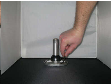
Remove Rotor O'Ring, clean & check condition
