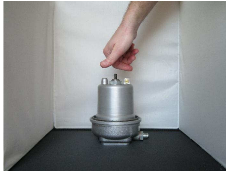
Spin Rotor with fingers to check for free rotation
