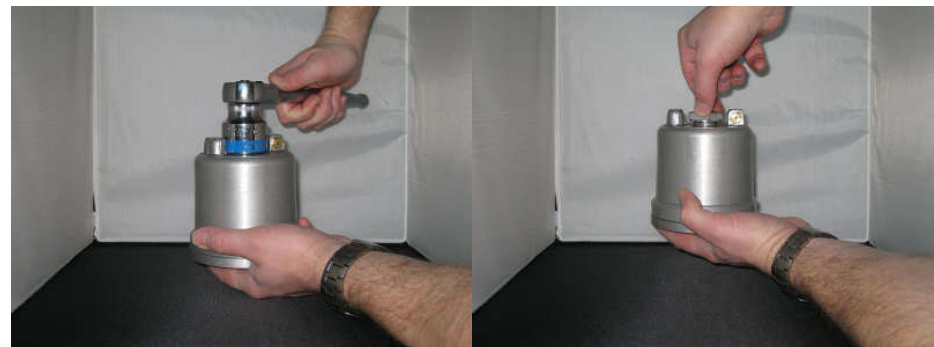
Remove Rotor Nut with 32mm Socket
