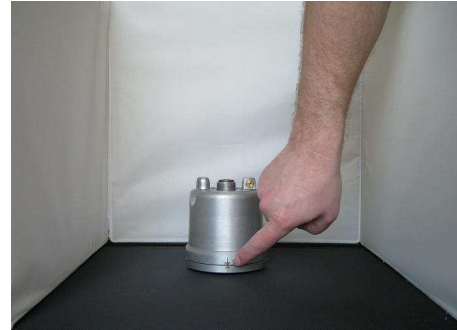
Line up Arrows on Rotor Cover and Base
